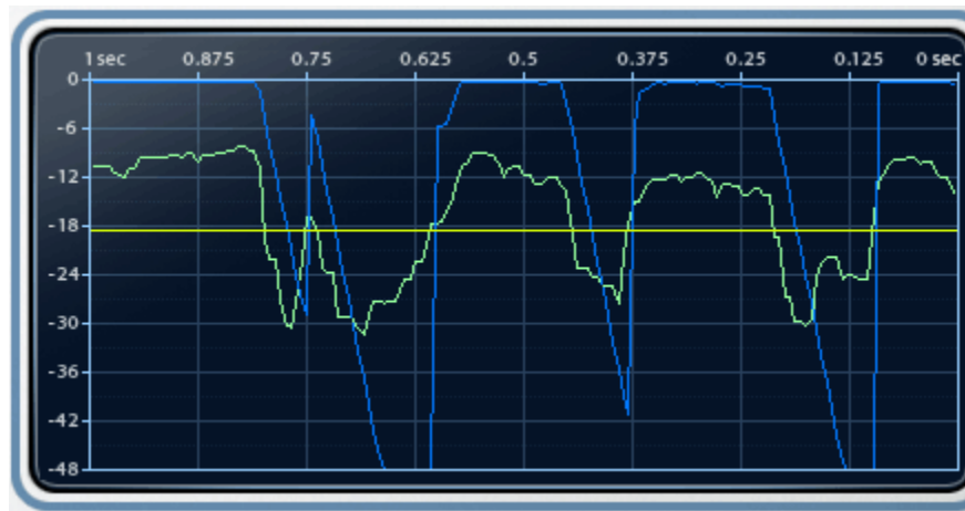
Figure 7-4. MR Gate time display. The green plot is the input signal level, the blue plot is the gate gain, and the yellow line is the threshold.
