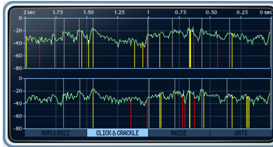
Figure 5-5. Click and Crackle event display. The green plot shows signal level, red lines are clicks, yellow lines are crackle, and grey lines are onset events.
