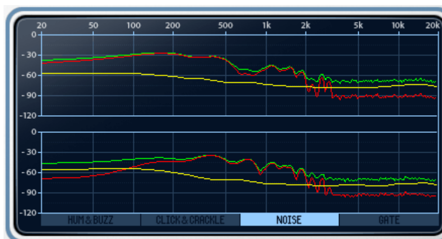
Figure 6-5. Noise reduction spectrum display. Green is input signal spectrum, red is output signal spectrum, and yellow is the noise floor spectrum. For stereo inputs, the left channel is displayed on top, and the right channel is displayed below.
