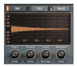
The envelope is a simple Attack/Hold/Release envelope with the following controls:
