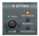
Normalize will automatically apply gain so that the wet reverb sounds equally loud as the dry sound. If Normalize is off, you can dial in the gain yourself using the IR Gain control. The IR Gain control has no effect if Normalize is enabled.
