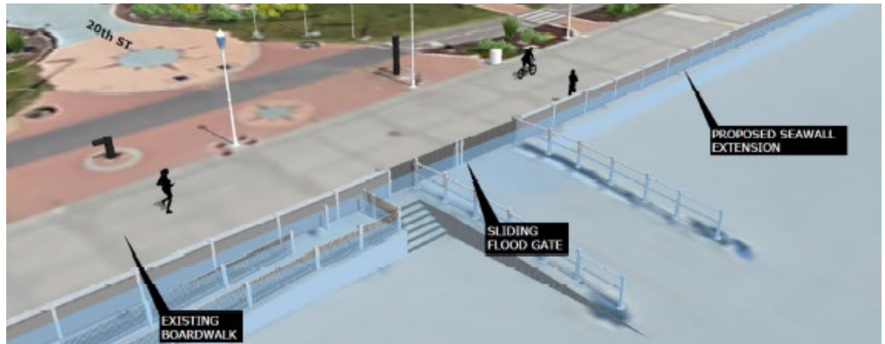
FIG. 4.2.26 RENDERING OF RAISED SEAWALL & SLIDING FLOOD GATE AT BOARDWALK Virginia Beach, Virginia
