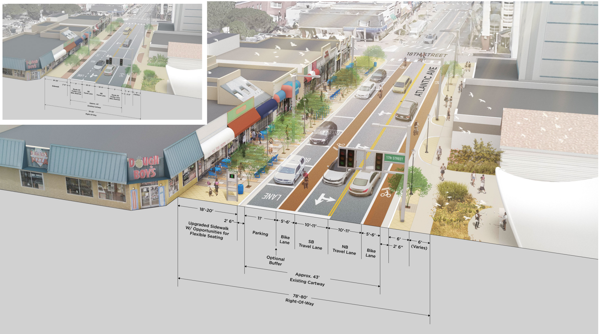
FIG. 4.2.34 ATLANTIC AVENUE AT 17TH STREET – EXISTING CONDITIONS (TOP LEFT) AND CONCEPTUAL INTERIM OPTION FOR FURTHER STUDY: Dimensioned street section — off-season (on-street parking and dedicated bike lanes)
