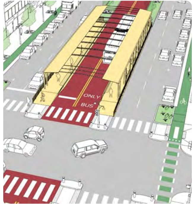
Figure 7-25 - Regional Multimodal Corridor Cross Section
