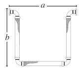
Class 150 carbon steel plate flanges, stainless steel corrugated hose, and single stainless steel braid (+/-2" axial).
