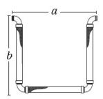
Schedule 40 carbon steel male NPT threaded ends, stainless steel corrugated hose, and single stainless steel braid (+ / -4"axial).
