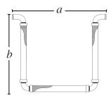
Schedule 40 carbon steel grooved pipe ends, stainless steel corrugated hose, and single stainless steel braid (+/-2" axial).
