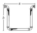
Class 150 carbon steel plate flanges, stainless steel corrugated hose, and single stainless steel braid (+ / - 8" axial).
