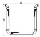
Schedule 40 carbon steel grooved pipe ends, stainless steel corrugated hose, and single stainless steel braid (+/-8" axial).
