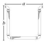
Schedule 40 carbon steel male NPT threaded ends, stainless steel corrugated hose, and single stainless steel braid (+/-2" axial).
