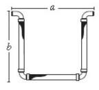
Schedule 40 carbon steel grooved pipe ends, stainless steel corrugated hose, and single stainless steel braid (+/-4" axial).
