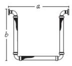
Class 150 carbon steel plate flanges, stainless steel corrugated hose, and single stainless steel braid (+ / – 4" axial).
