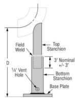
Fig. 62 Stanchion with adjustable base.
