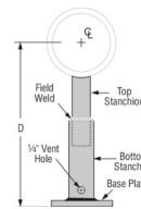
Fig. 62 Type B (S.R. Elbow) with Adjustable
