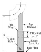
Fig. 62 Type A (L.R. Elbow) with Adjustable
