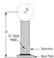
**Fig. 63 Type C Horizontal Pipe**
