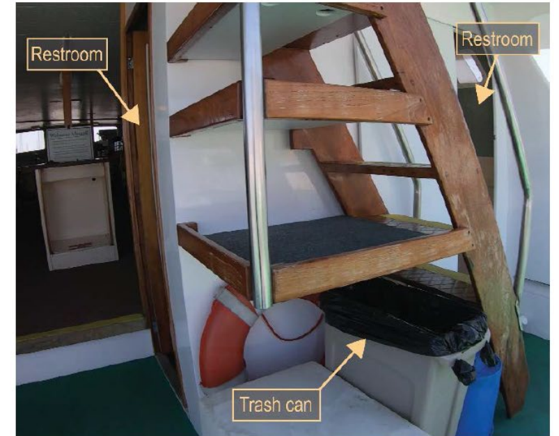
Figure 18. Left: Photo from a previous voyage of stairway to the upper deck and restrooms of the Conception . Note the regular stowage of a polyethylene trash can under the stairway aft of the salon. Right: Still image from a 2019 video taken of the stairway on board the Conception with shelving installed. (Source: M. Ryan [left], R. Clevenger [right])
