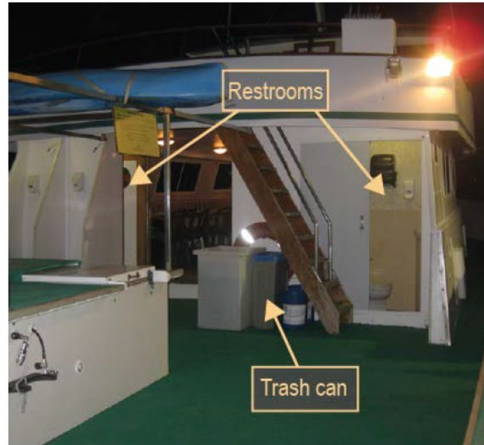
Figure 18. Left: Photo from a previous voyage of stairway to the upper deck and restrooms of the Conception . Note the regular stowage of a polyethylene trash can under the stairway aft of the salon. Right: Still image from a 2019 video taken of the stairway on board the Conception with shelving installed. (Source: M. Ryan [left], R. Clevenger [right])
