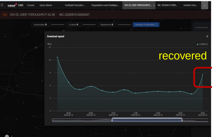
Performance issue auto closed after the throughput KPI such as the download speed returned to normal level.
