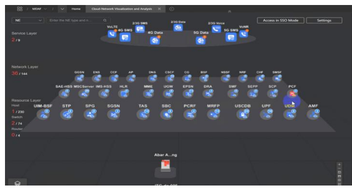
VNF object (5GC NFs and EPC VNFs) status (faulty or normal) visualization
