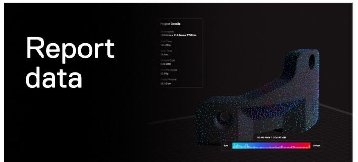
View the deviation across the part's geometry, and set tolerance limits to assess part quality. The print report is saved in Eiger and can be referenced at any future date.
