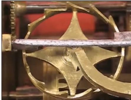
This verge escapement is part of a clock built nearly two centuries after Huygens’s; we are looking down upon the crown wheel. Notice how the pawls are brought alternately to bear against opposite teeth. Each quarter-turn of the axle corresponds to a half-swing of the pendulum. By the way, the verge escapement takes its name from this axle, called the “verge” from Latin *virga*, a rod or stick.
