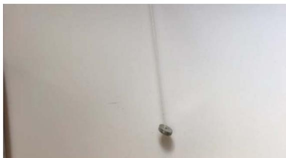
each swing has noticeably decayed. *Now* the time for the same number of swings is 6.17 seconds, or 1.234 seconds per swing. Not quite equal, but certainly very close. We will ask later on whether the difference is significant. For now, though, it appears that every undulation of the pendulum occupies pretty much the same interval of time, without regard to the size of the swing. This is the property called *isochrony*.
