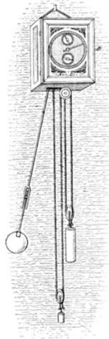
clocks achieved far greater accuracy than did earlier clock mechanisms. But was that improvement due to the *isochronous path* of the pendulum, or to the *pendulum* itself, regardless of path?
