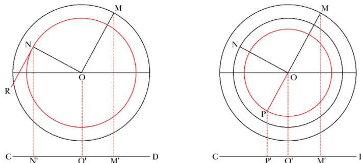
is, the rate of change of ON, while ON in turn is the velocity of M. Then OP is the rate of change of the velocity of M—it is the *acceleration* of M.
