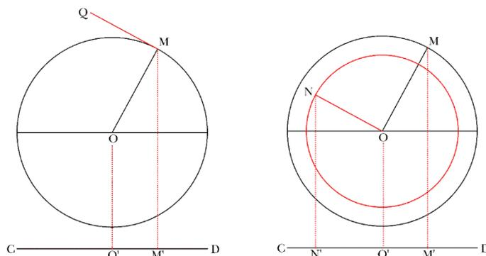
length). Then draw ON equal and parallel to MQ. Thus it is clear that ON, likewise, represents the velocity of point M.
