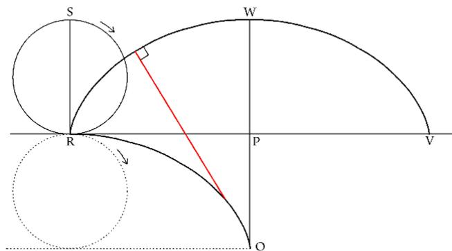
He then proves that any tangent to the lower cycloid cuts the upper cycloid at right angles. That perpendicularity is the property which enables a suspended body to swing in a cycloidal curve, as we can see by inverting the picture.
