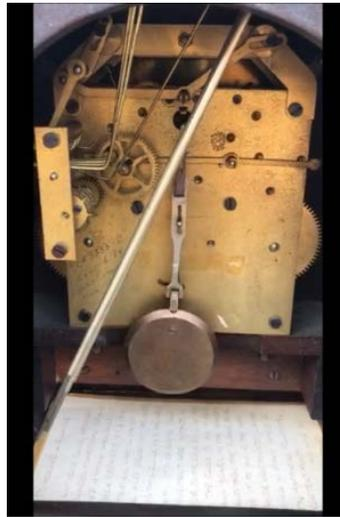
The pendulum is mounted on a ribbon of spring brass, which eliminates the friction and wear of a pivot and bearing, while being weak enough to exert negligible effect on the pendulum's period. The period of this model is .723 seconds.
