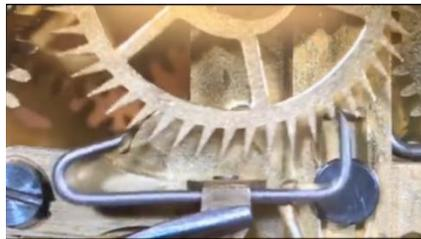
I hope you can see how the angled ends alternately stop, and are then pushed out of the way by, successive teeth—each time receiving a nudge that is transmitted to the pendulum. That escapement was widely employed in mantel clocks like this one:
