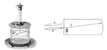
instrument balanced the tension between two electrified spheres against the elastic twist of a slender thread—just as our modern electrometer, as in the diagram we saw earlier, balances the tension between two electrified plates against the elastic stretch of a spring. Both instruments, therefore, serve to measure electric tension.
