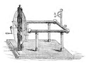
electrometer mounted on the prime conductor; this was one of the chief applications of the Henley device.
