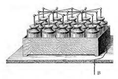
conductors, which are connected to the jars' inner coatings, are all joined together. Within the wooden container, the outer coatings rest upon a conductive plate that is connected to the flexible chain B, which in turn is connected to the earth.
