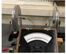
And again we connect Capacitor A to the Wimshurst machine, and charge it to an initial tension.... Its electrometer reads 2.83 units, nearly the same as before, while of course the other electrometer continues to read *zero*.
