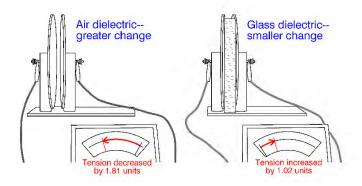
• Thus one and the same quantity of electricity is associated with *lower tension* when the dielectric is glass, and *higher tension* when the dielectric is air.
