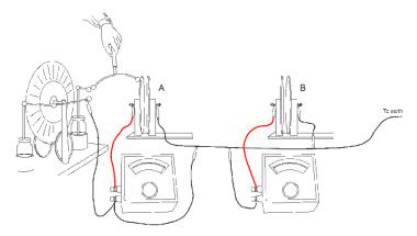
approaches its full scale reading. Capacitor A will thus sustain a definite tension, indicated by the electrometer. Capacitor B, of course, will remain uncharged and will sustain *no* electric tension.
