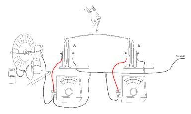
what must happen when I do that. The joining wire is a good conductor, so it cannot
