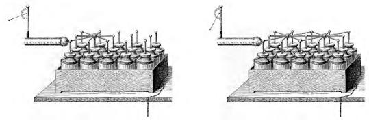
But our experiment, like Faraday's in the Eleventh Series, compares the tensions of different quantities of electricity in one and the same capacitor. The two experiments are not comparable, because in the earlier exercise the physical environment underwent significant change—from a smaller number to a greater number of jars—while in the later experiment the environment did not change: the electrometer measured the variation of tension in one and the same capacitor.
