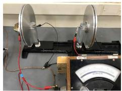
Here is the setup. The copper wire that is appearing on the left will connect capacitor A to the Wimshurst machine... Now I am cranking the machine, and you can see the electrometer rise almost to its full scale.
