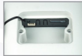
Detail of MicroSD Card Slot
