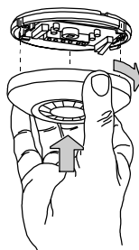
Figure 3 – Installing the Cover
