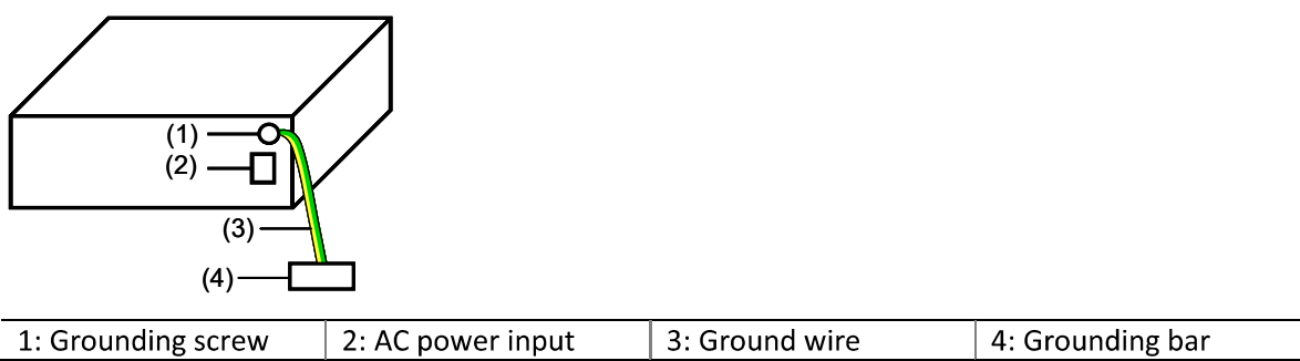
Figure 4-6 Ground the device through a grounding bar
