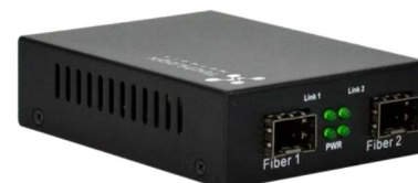
TL-MC-1S1S 1G media converter with dual fiber ports. Ideal for converting multimode to single mode or duplex to simplex when using compatible SFP modules.
