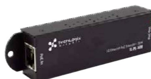
TL-PE-30W Extends 30W PoE beyond the 100m maximum distance. Up to 5 units may be cascaded.
