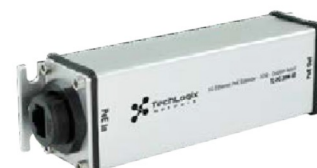
TL-PI-30W-IO Extends 30W PoE beyond the 100m maximum distance. Up to 5 units may be cascaded. Supports outdoor installation and harsh environments.
