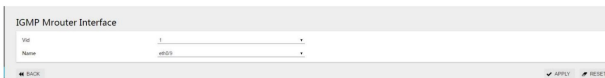
Figure 3-92 IGMP routing interface configuration
