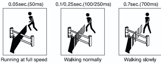
Function setting switch (Factory setting : 0.05sec.)
