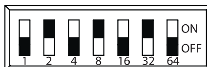
FIGURE 14: Enlarged View of PAD Device with Dip Switch Setting Addressed
