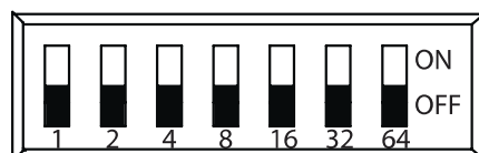
FIGURE 13: Enlarged View of PAD Device with Dip Switch Setting Unaddressed
