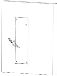
Figure 3-38 Cave the Installation Hole
