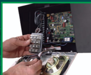
Modular Design makes installation and service easy
