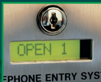
1810 Built-in Display Indicates door/gate has been opened
