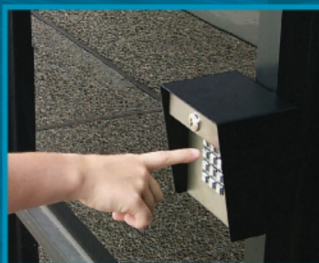
Keypad Users enter a unique PIN to gain entry
