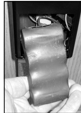
FIG. 18: INSERT BATTERY PACK INTO HOUSING
