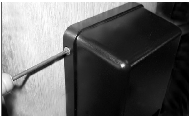
FIG. 16: SECURE TOP OF INSIDE HOUSING
