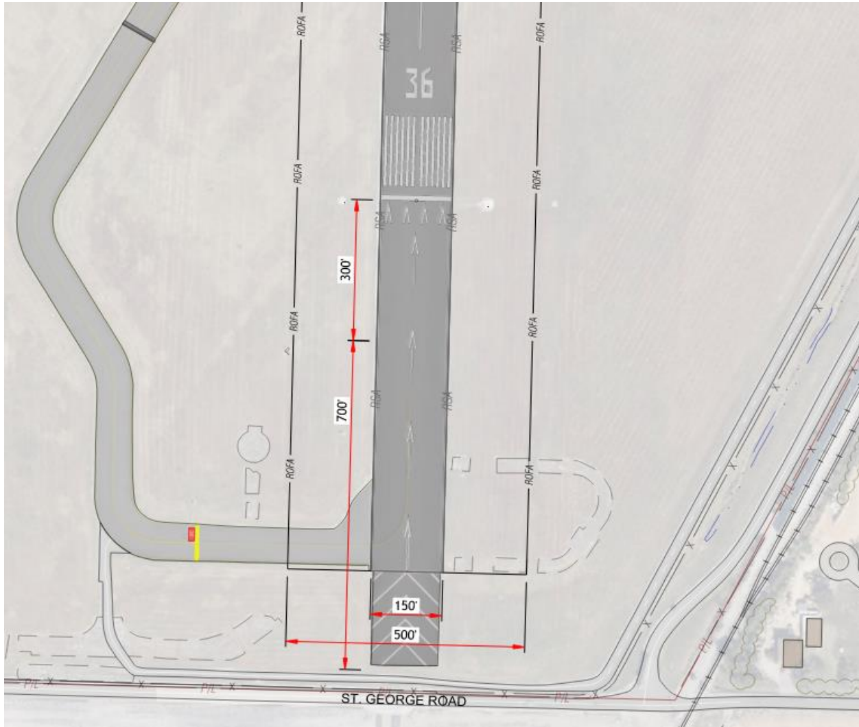
Figure 4-8 – Existing RSA/ROFA (Runway 36 Approach End)
