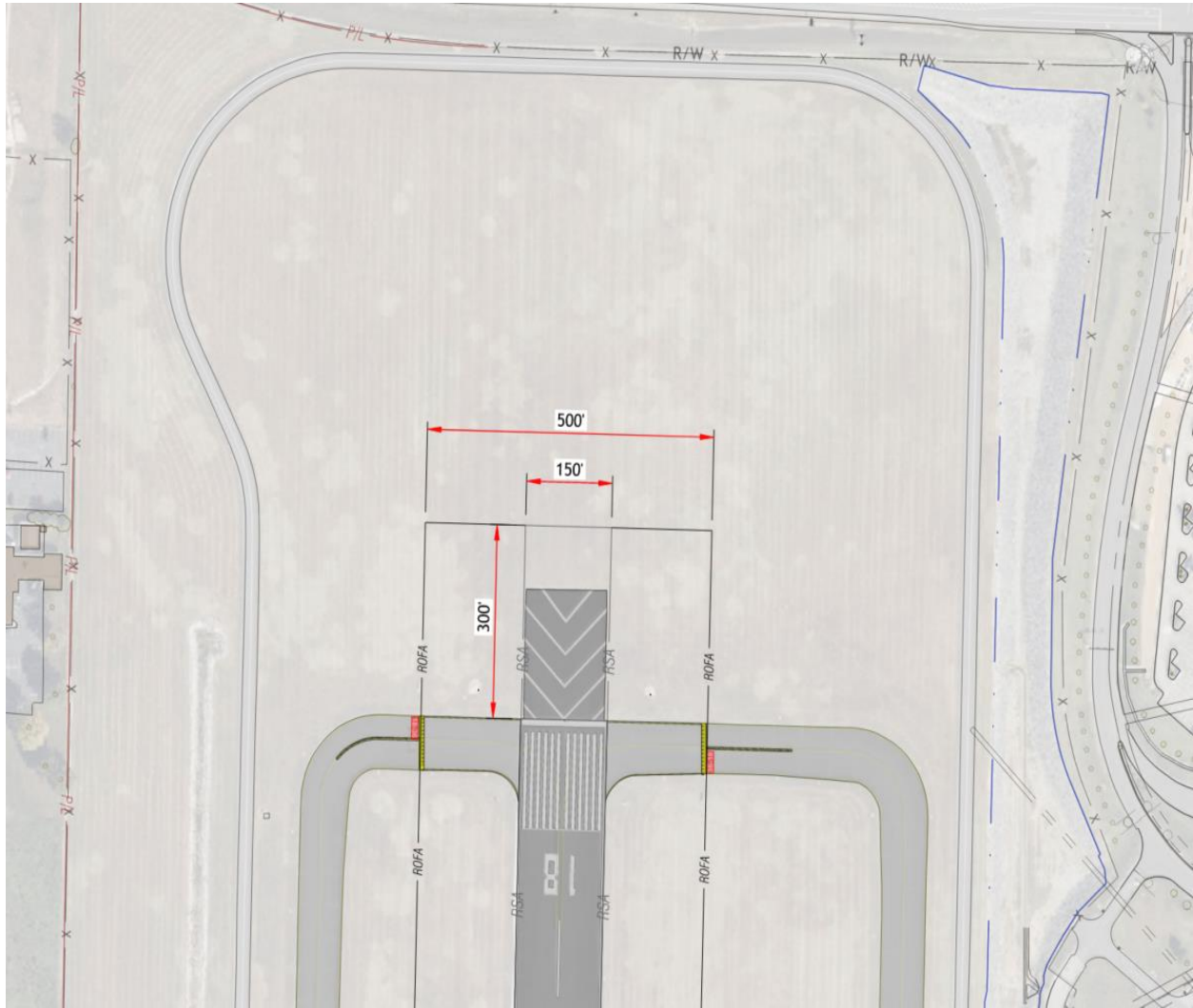
Figure 4-10 – Existing RSA/ROFA (Runway 18 Approach End)
