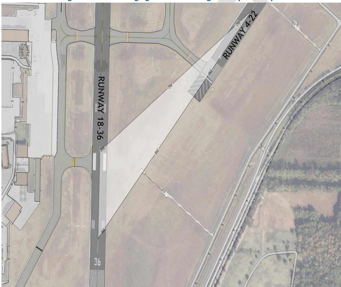
Figure 4-22 – Converging Non-Intersecting Runway Visibility Zone
