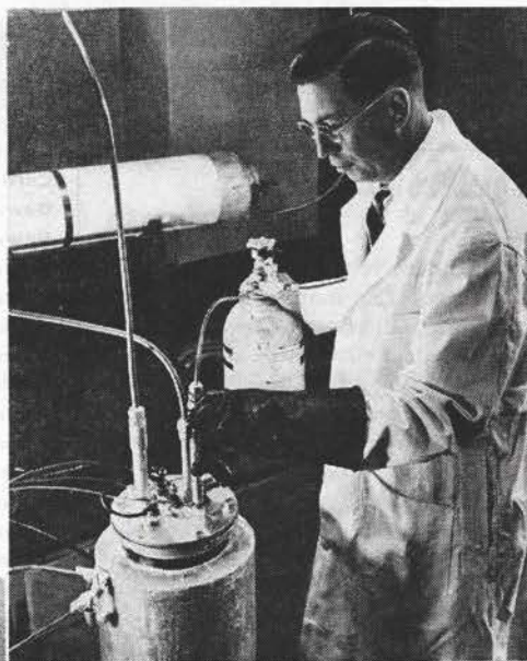
Above. Laboratory fluorine cell and a spare cell head. Note symmetry of anode, screen diaphragm, and perforated cathode. Such a cell is capable of producing approximately 20 liters of fluorine an hour
