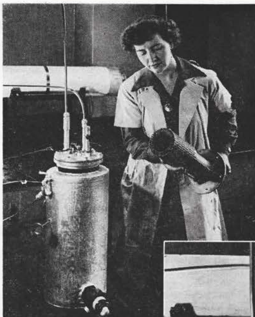
Above. Laboratory fluorine cell and a spare cell head. Note symmetry of anode, screen diaphragm, and perforated cathode. Such a cell is capable of producing approximately 20 liters of fluorine an hour
