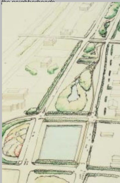
Open spaces in a sustainable suburban corridor create the green infrastructure to manage storm water and non-point source pollution
