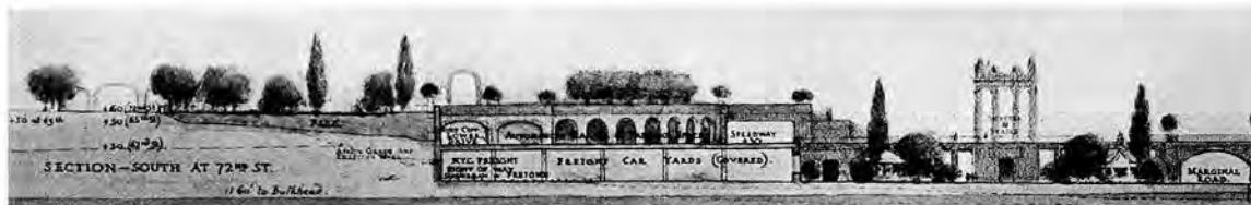
CROSS SECTION AT 72ND STREET, INDICATING THE POSSIBLE DISPOSITION OF VEHICULAR AND RAIL TRAFFIC
