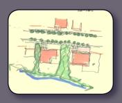
Tree grid and pervious paving turns parking lots into multi use space
