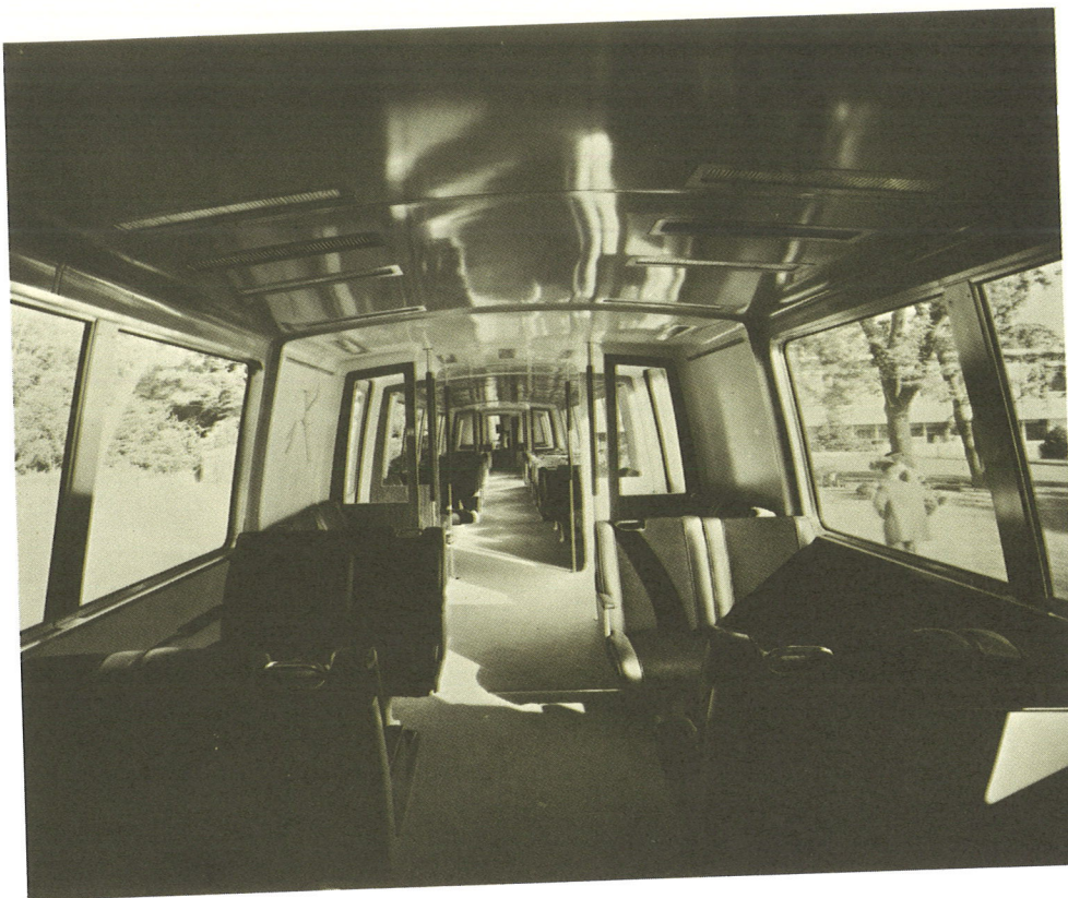
"The most luxurious interior ever provided for a rapid transit vehicle," according to its prospective manufacturer, General Steel Industries. This car was designed for the Bay Area Rapid Transit District. It will be air conditioned, have a new type of suspension and run on resilient, all-welded rails to provide more comfort and quiet than present rail transit lines do.
