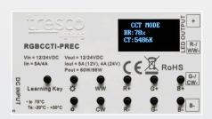
Digital readout allows precise tuning of the color temperature from 2700K-6500K & brightness control.
