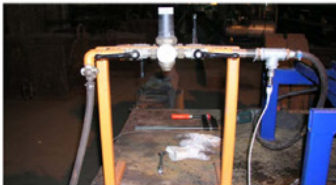
Pressure control with Manometer
