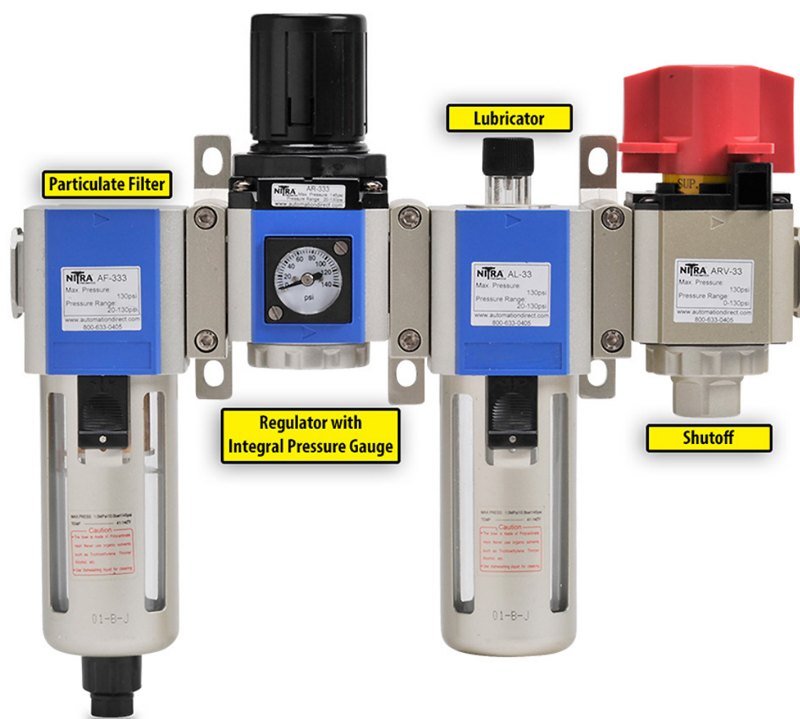
Figure 10A: Basic Air Prep System
