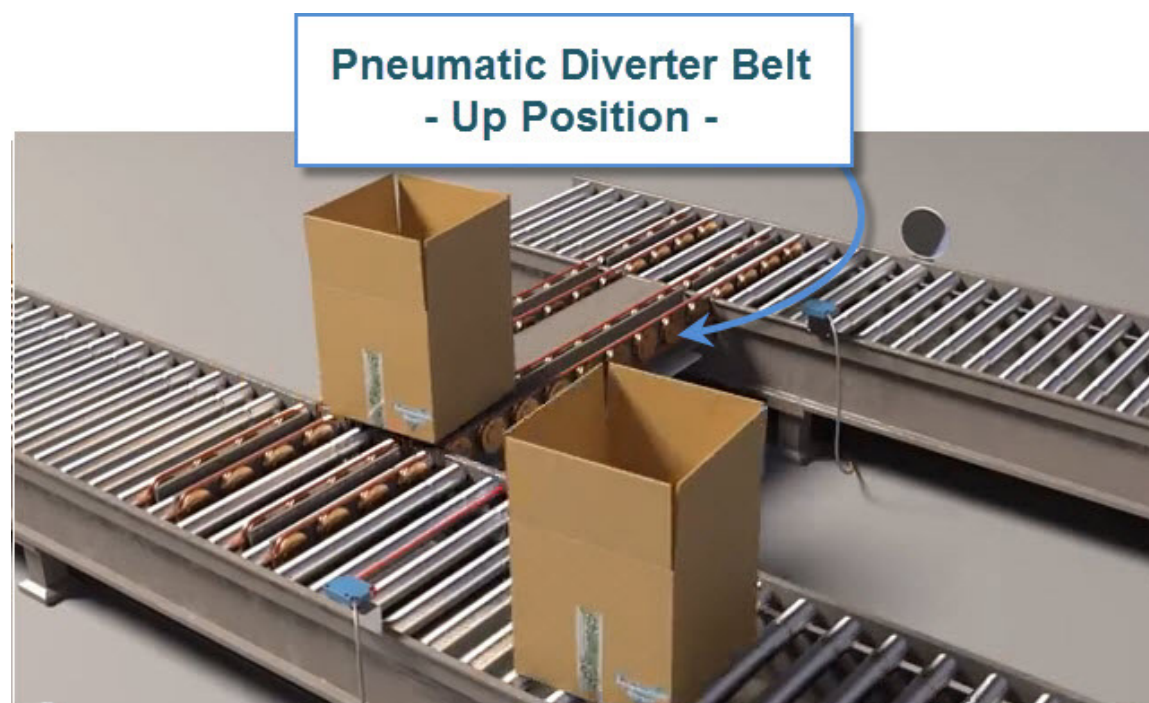
Figure 9B: Pneumatic diverter belt, up position
