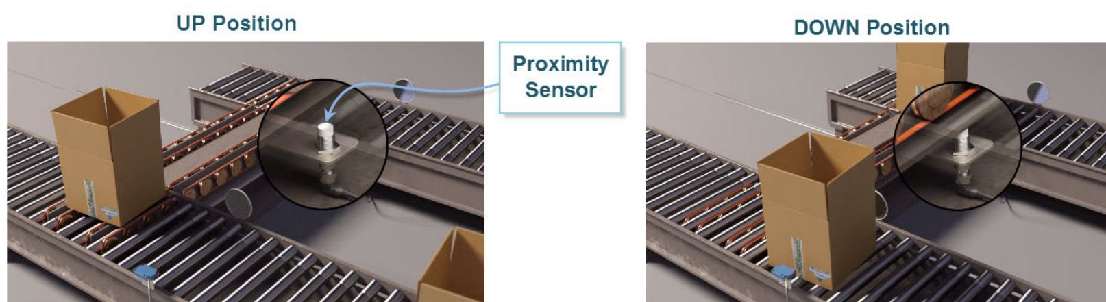
Figure 9H: Proximity sensor example
