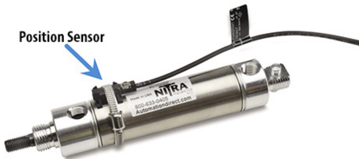
Figure 9G: Typical installation of a position sensor on a cylinder with a magnetic piston
