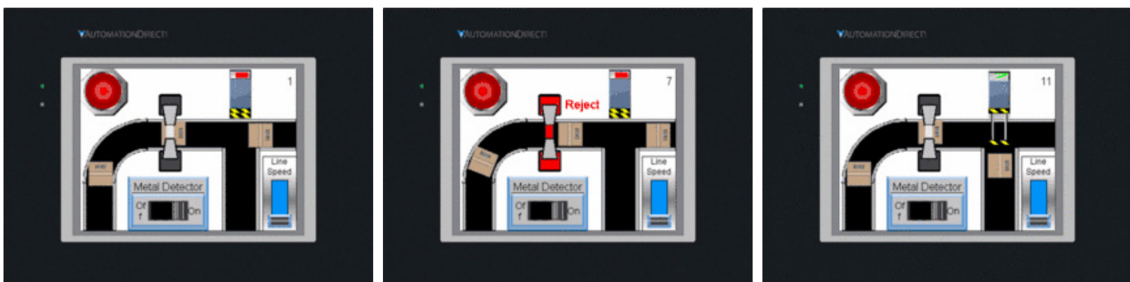
Figure 1B: Simple pneumatics application: Air cylinder powered ram to divert rejects to another conveyor
