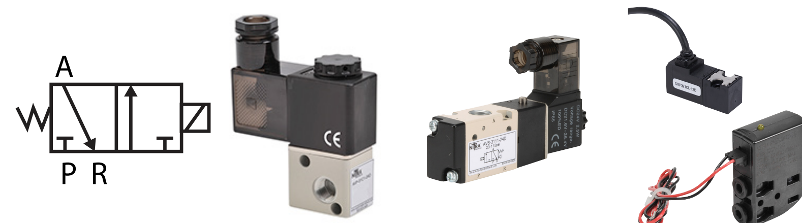
Figure 5C: 3-Port (3-way), 2-position, normally closed solenoid valve, spring return
