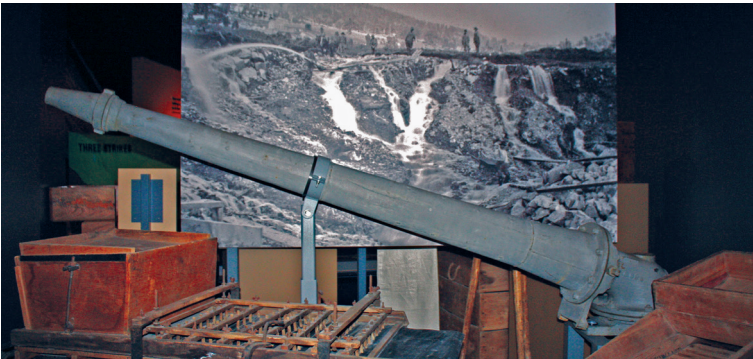
A huge hose nozzle used to wash gold from the sides of mountains fills this display. Diamond City, in Confederate Gulch on Canyon Ferry’s east side, was totally washed away by hydraulic mining. MT43 News Photo
