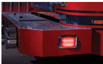
FireRay LED 6x4 (FR6C1-R) mounted on bumper with two-to-four hole conversion kit (FR6-A4HMC)
