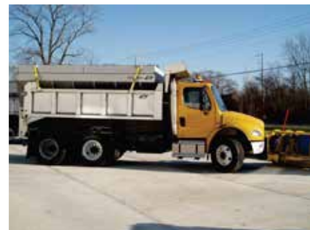
Figure: 14' WXL body and E/AC Spreader in 304 SS
