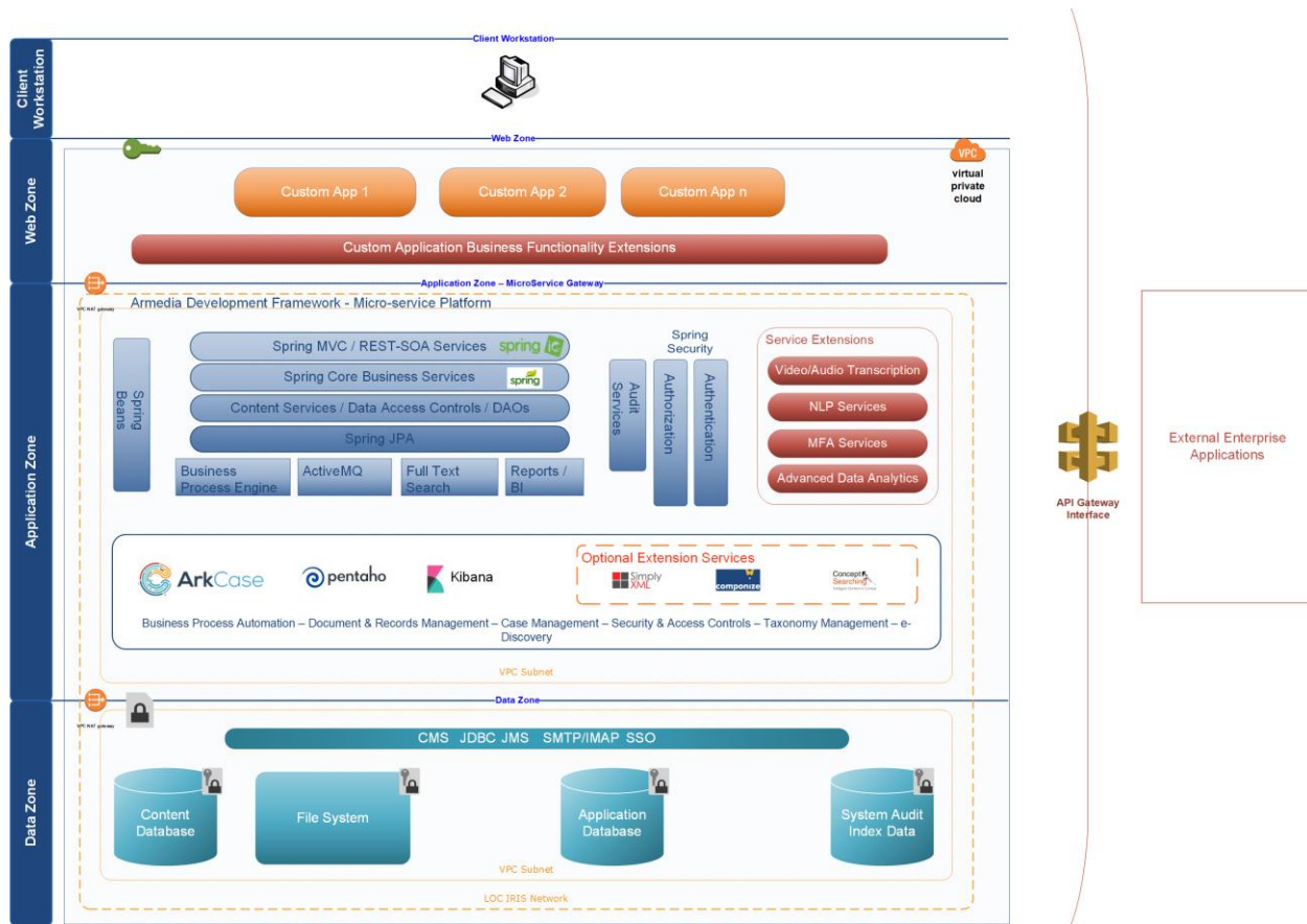
Figure 5 - Armedia Development Framework - Framework for extending ArkCase and create specific business extensions as needed
