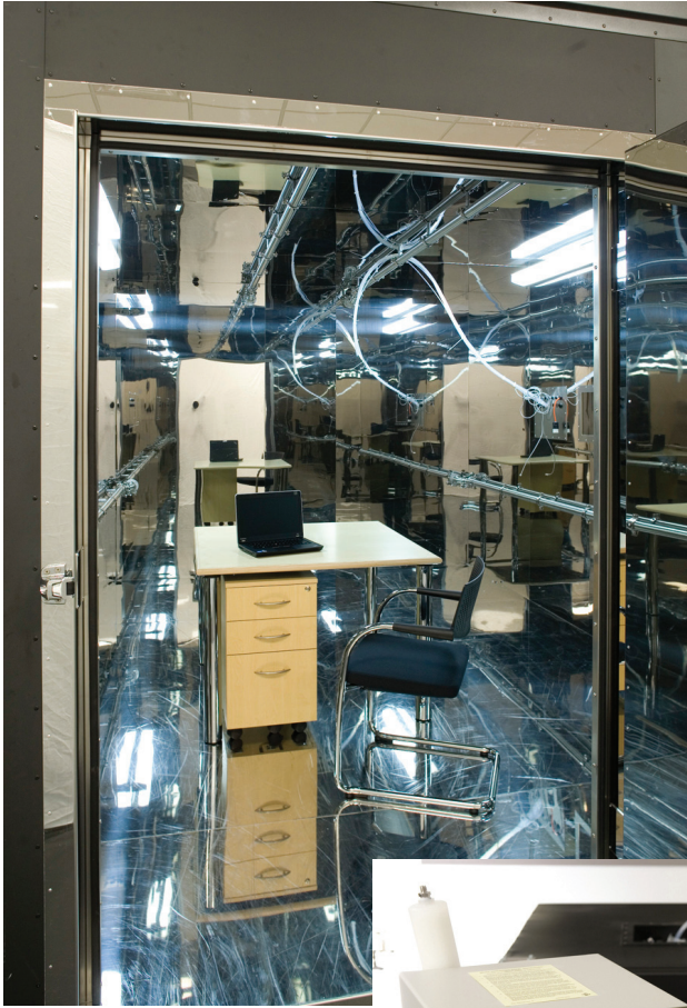
Stainless steel dynamic environmental chambers are used to test products for indoor air emissions. Each chamber maintains a constant temperature, relative humidity and ventilation rate. (Photos courtesy of Air Quality Sciences, Inc.)
