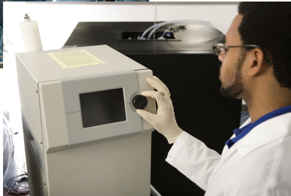
Stainless steel dynamic environmental chambers are used to test products for indoor air emissions. Each chamber maintains a constant temperature, relative humidity and ventilation rate. (Photos courtesy of Air Quality Sciences, Inc.)
