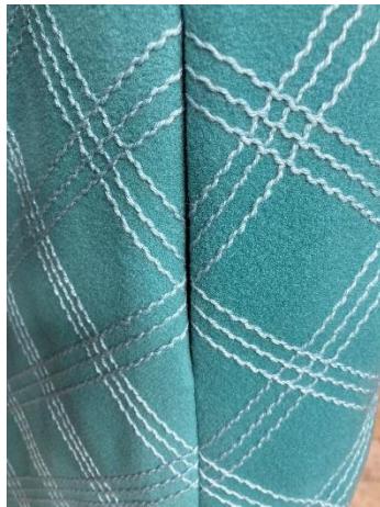
Sleeve front and back basted to check alignment and then stitched.
