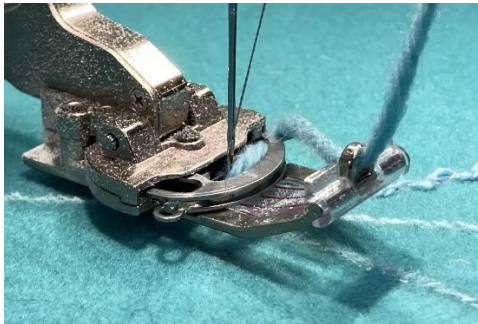
With the needle up and wipers closed, raise the presser foot and turn the fabric. Align the marking on the insert and lower the presser foot. Stitch to the top of the "V".
