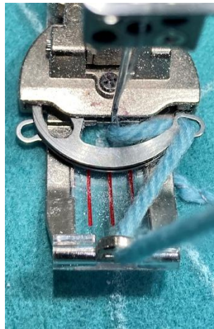
With the needle up and wipers closed, raise the presser foot and turn the fabric. Align the marking on the insert and lower the presser foot. Stitch to the top of the "V".
