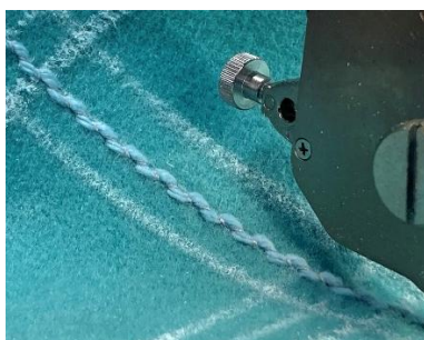
Stitching on center marked line on each set of markings before stitching on the second marked line.
