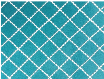
Single row of stitching – using an off-white yarn.
