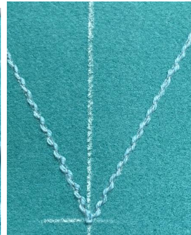
With the needle up and wipers closed, raise the presser foot and turn the fabric. Align the marking on the insert and lower the presser foot. Stitch to the top of the "V".
