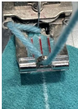
Alignment of center mark on insert with marking on fabric.
