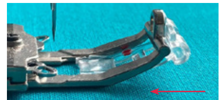
First position when inserting 5mm Cording Micro Insert foot
