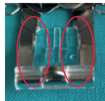
Alignment position for Micro Insert Foot
