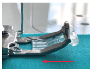
First position when inserting micro insert
