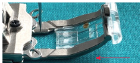
First position when inserting micro insert foot
