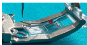
Micro Insert Foot in final position
