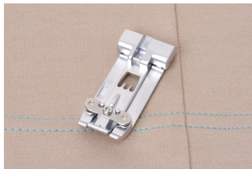
Point Ourlet Couvert Large sur tissu tricot, S.L. 4.0.
