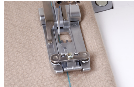
Alignment of the C1(left) needle with the raised notch on the Compensating Foot with the markings on the fabric.
