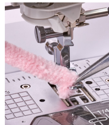
#6/#7 weight yarn inserted in 5mm couching foot and Yarn Guide.
