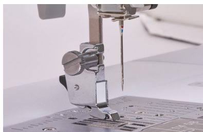
Presser foot in the lowered position.
