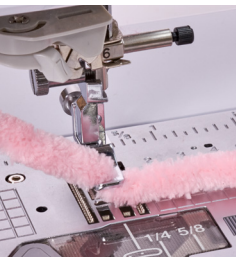
#6/#7 weight yarn inserted in 5mm couching foot and Yarn Guide.
