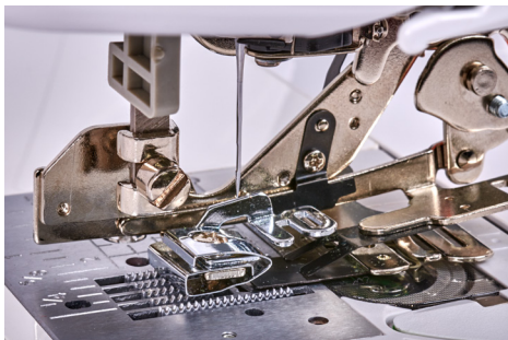
Guide in position on presser foot bar.
