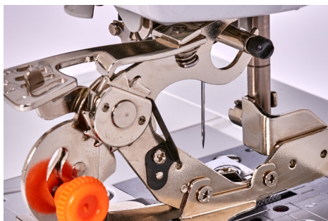
Fork (u shaped) Guide in position with the Needle Clamp Screw.
