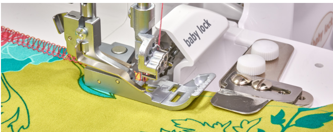
Stitching 4-thread overlock stitch with decorative thread in each looper and overlock thread in the needles.
