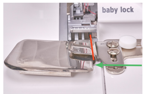
\frac{1}{4} " Single Downturn Feller attached to the Compact Overlock Table.
