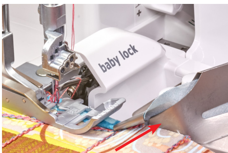
Fabric base positioned in guide and attaching fabric strip.
