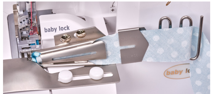
Fabric strip inserted into the binder attachment with the wrong side facing forward.
