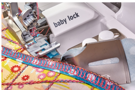
36mm Double Fold Bias Binder, 4-thread overlock with 12wt. cotton in the upper and lower loopers.
