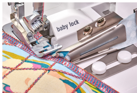
10mm Knit/Woven Double Fold Bias Binder, 4-thread overlock with 12wt. cotton thread in the upper and lower loopers.
