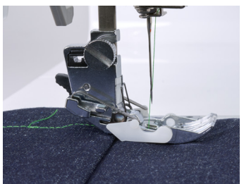
Presser foot at the end of stitching off the seam and back onto the flat part of the hem.
