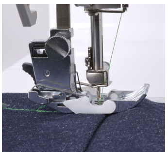
Presser foot levels out moving across the top of the seam.
