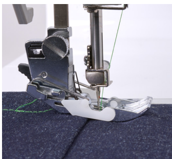
Presser foot changes to a downward angle as stitching continues down the seam.
