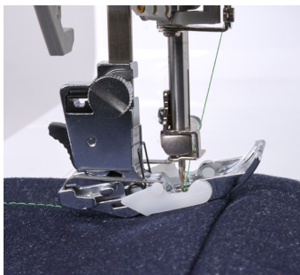
Presser foot angle adjusting to navigate the change in fabric thickness (bulk of seam and hem).
