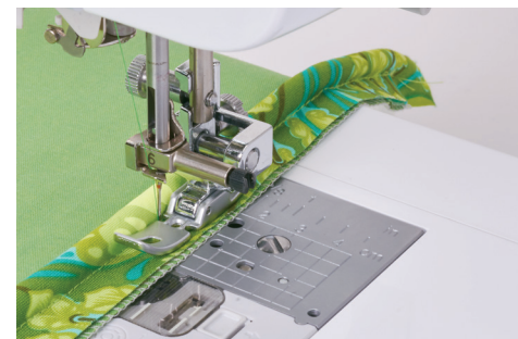
Attaching piping to fabric.
