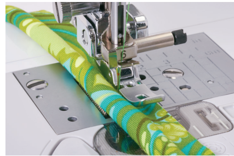
Wrapped cording under the presser foot with the presser foot and needle aligned with the cording.
