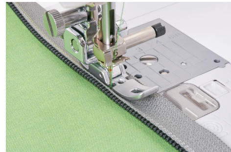
Fabric and zipper coil to the left of the presser foot and needle.
