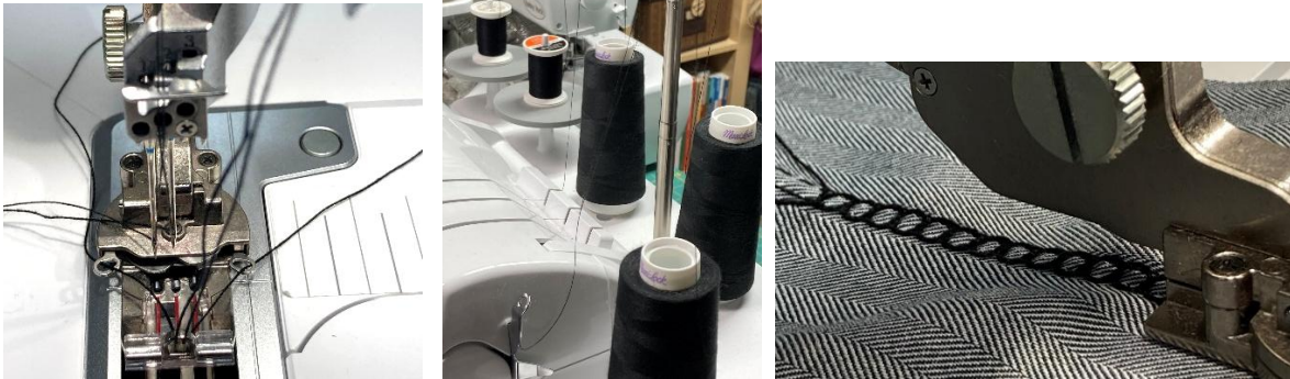
Wipers threaded with 12wt. thread with overlock thread in the C1/C2 needles and chain looper and my test stitch sample.
