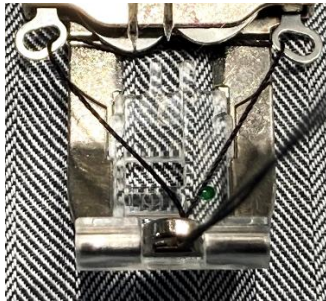
5mm Taping Micro Insert in position on the combination foot with the ribbon place in the first guide, then the second with the final step testing the ribbon position with the C1 & C2 needles.
