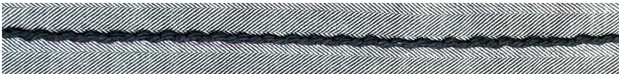
Stitch for the hem; Top Cover Chain Stitch – stitch length of 3.0 using the cotton yarn.
