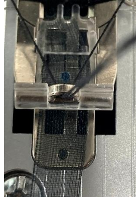
8mm Taping insert in position on the combination foot.
