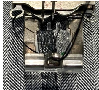
5mm Taping Micro Insert in position on the combination foot with the ribbon place in the first guide, then the second with the final step testing the ribbon position with the C1 & C2 needles.
