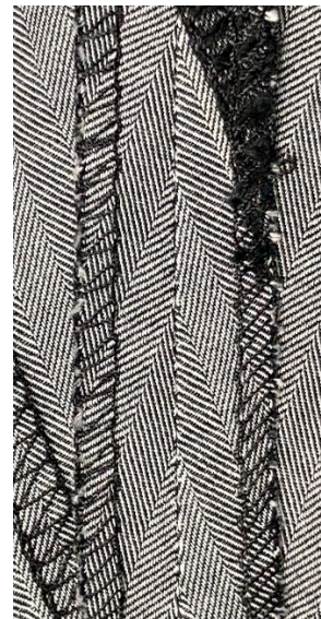
3-thread overlock narrow to finish fabric edges, straight stitch seam with seam pressed open.
