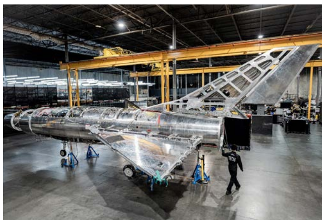
Figure 12: Hermeus Quarterhorse Mark 2 Under Construction
