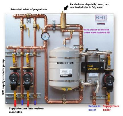
**5. Connect Manifold to Pump Panel:** Connect your manifold to the pump distribution panel using copper or PEX piping. The threaded fittings below will attach to the supply/return ball valves on your manifold, while the straight couplers will connect to the supply/return lines on the pump distribution panel.
