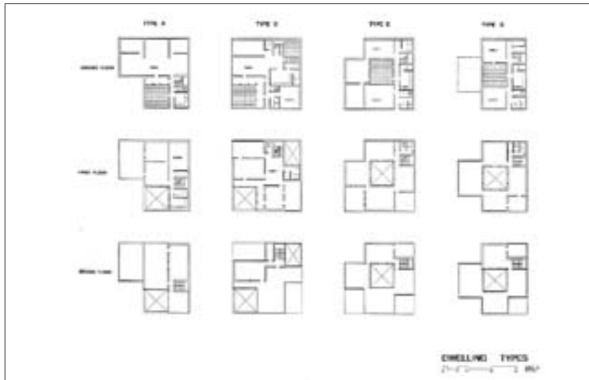
Figure 7: The four dwelling types that were used in the test design. The drawing assumes that each dwelling is built up to its maximum three stories (Source: author).
